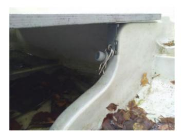
In the front bottom part of the boat there is a hole for water flow. A special cork closes it. If the hole is open, the cork hangs by the side, as shown in the picture.
